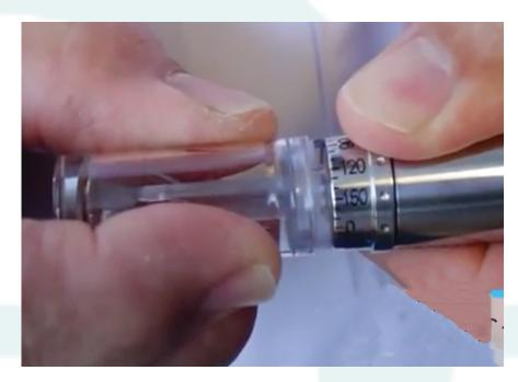
4. Align the RoboTip<sup>™</sup> to the axis dial and remove cap.
